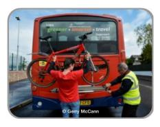
Stagecoach Highland was keen to take part and funded the installation of the racks themselves in the summer of 2013. Stagecoach developed a low cost system effectively mounting a typical wheel supporting bike rack as you would use on a normal car, which can carry up to three bikes. They put a booking system in place so that people had the option of booking the bike on in advance to ensure space was available. The racks are removed in the winter to extend their life.
